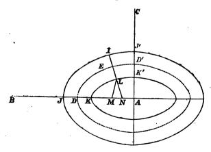
lines KK', JJ', DD', respectively. The eye is supposed to be situated on the axis OA, viewing the sphere from a considerable distance. All great circles on the sphere are represented by straight lines. Since the cones are co-axial with the momental ellipsoid, these sphero-conics are symmetrical about the principal planes of the body. The intersections of these principal planes with the sphere will be three arcs of great circles, and the portions
